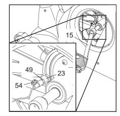
Slide the Reed Switch slightly closer to or away from the Magnet. Then, retighten the Screw. Turn the Left Crank Arm for a moment. Repeat until the console displays correct feedback. When the Reed Switch is correctly adjusted, reattach the left Pedal Guard (8) and the left Side Shield Cover (14).
